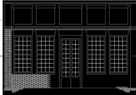
Figure 2. Based on the evidence, this drawing indicates the Garden House measured 21 ½' tall by a little over 33' wide, with 9 ½'-tall windows—a grand structure consistent with European garden houses of the period.
